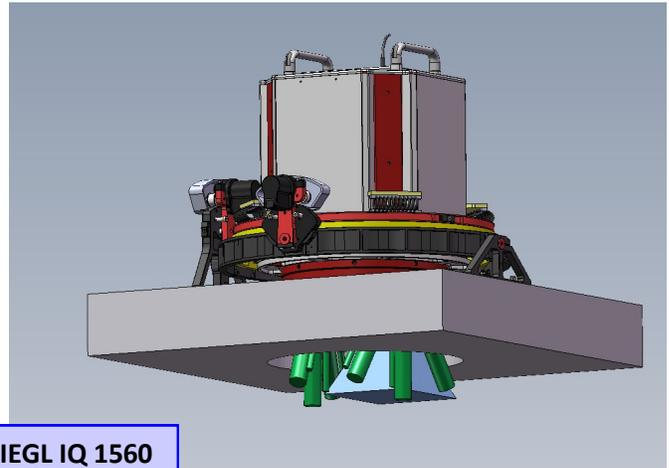
Contrary to other mount designs, the STX open circular gimbal allows the sensor system to be fixed into the mount so as to be as low as possible above the airplane hole. As the center of rotation is also located as low as possible, the scanner can take full advantage of the +/-10 degrees full range of correction in pitch and roll and +/-25 degrees of drift correction.
