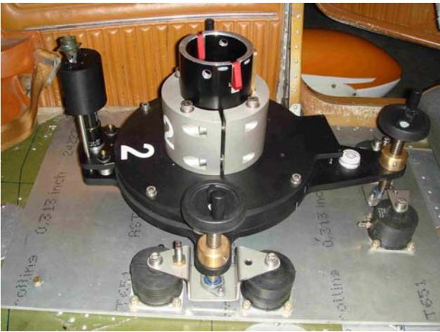
The mount installed in a Cessna 172 (USA)
